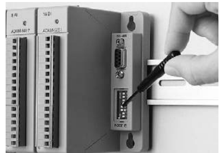
Node ID Setting 8-pin dip switch configuration
