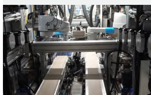
Stack welding machine
